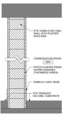
2 EXISTING 2-HOUR RATED FIRE COMPARTMENT WALL
